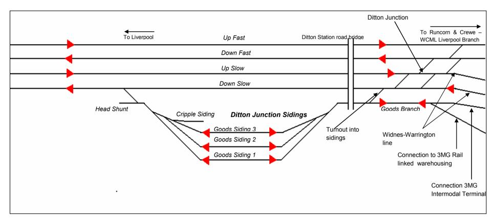
Not to Scale. The red arrows indicate direction of signalling on each line. Arrows pointing in opposite directions on a line indicates bi-directional signaling.
